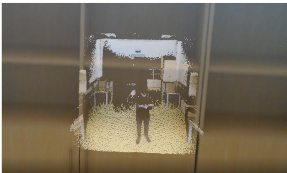
Obr. 4.4: Point cloud s hĺbkou 6m.
