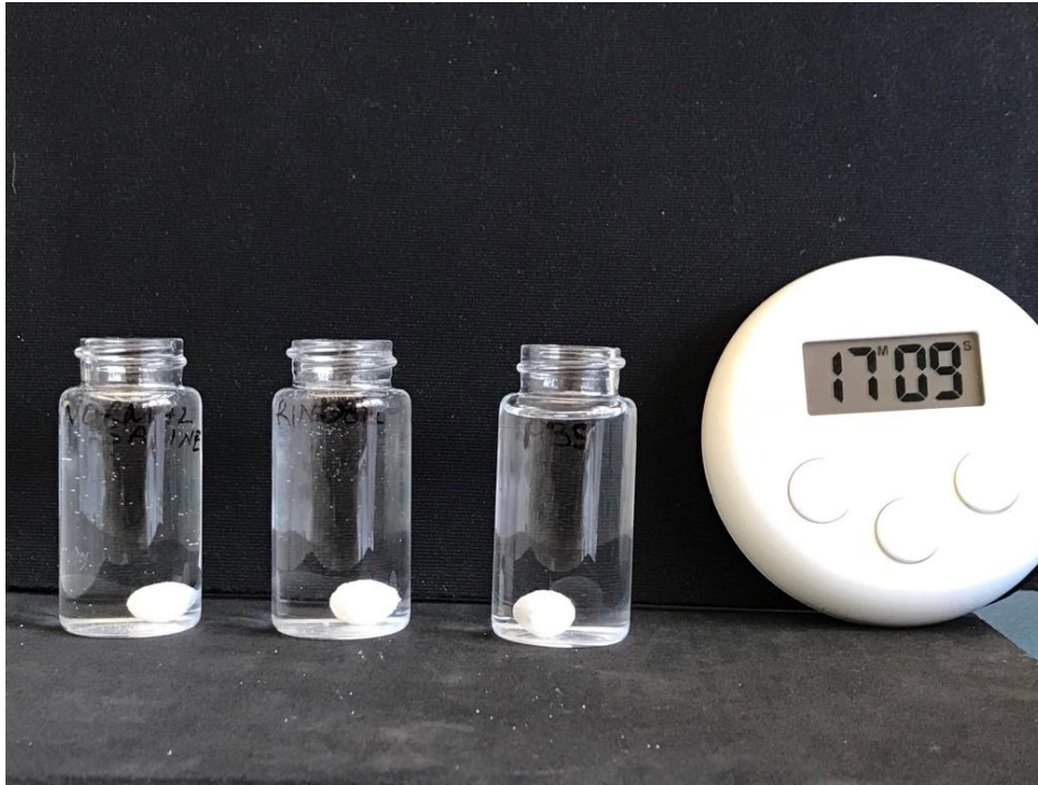
Figure 15: Washout resistance testing. 5 mm diameter balls immersed in normal saline, Ringer's, and phosphate buffer saline solutions. No sign of disintegration is apparent.
