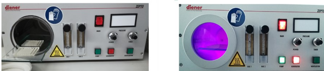
Figure 21: Oxygen plasma cleaner used to treat silicon platform in off and on state.
