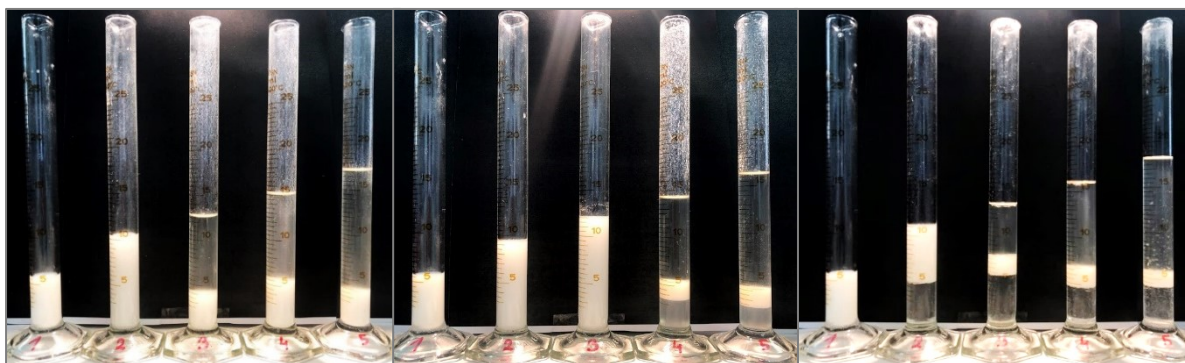
Figure 13. Photograph of salting-out induced phase separation and deproteinization of 50% milk solution. A: ACE used for deproteinization, 3 mL of mixed solution B added for salting-out. B: PrOH used for deproteinization, 4 mL of mixed solution B added for salting-out. C: MeCN used for deproteinization, 4 mL of mixed solution B added for salting-out. Cylinders numbered 1: control sample, 2-4: increasing solvent to milk solution volume ratio (2.5/5.0, 5.0/5.0, 7.5/5.0, 10.0/5.0 mL).
