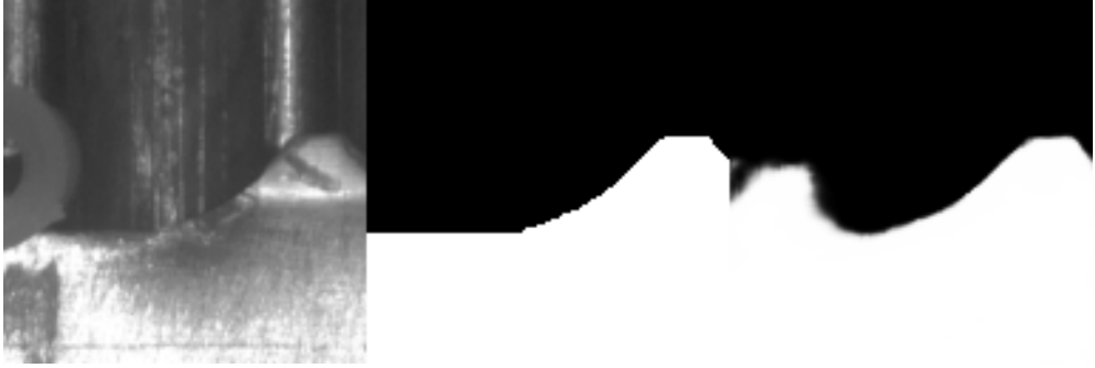
Figure 4.21: A problematic input for the Hard + debris dataset's model. The image is made of three sub-images: the left is the input, the middle is the expected mask and the right is the prediction.
