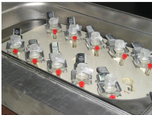
Figure 10 : FDC in the heating/stirring module
