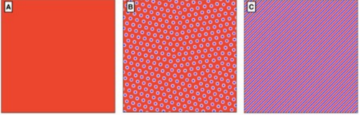
Figure 1.1. Out-of-plane ( z ) projection of the three main phases as shown on the bwr python colourmap (dark red corresponding to 1, dark blue corresponding to -1). A) ferromagnetic phase B) skyrmionic phase C) spiral phase.
