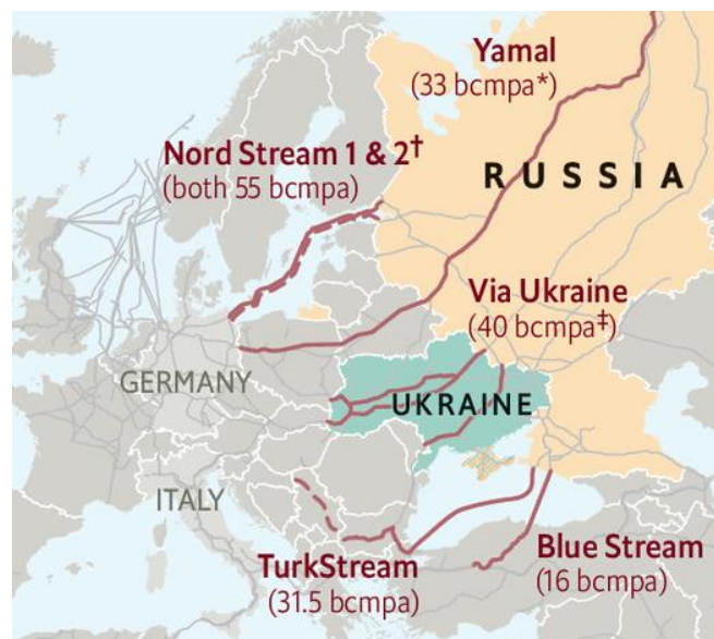
Figure 2: Capacities of the largest gas pipelines between Russia and Europe | Source: Bocksch (2022)
