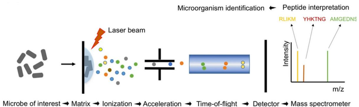
**Fig. 9 Diagram for mass spectrometry.** Three main components are included in a mass spectrometer: an ion source to form ions (ionization) and transfer them into a gas phase, a mass analyzer is the component of the mass spectrometer that takes ionized masses and separates them based on mass to charge ( $m/z$ ) ratios and outputs them to the detector to record the number of ions at each  $m/z$  value. Adapted from Sharma A. *et al.* (2020) [73].
