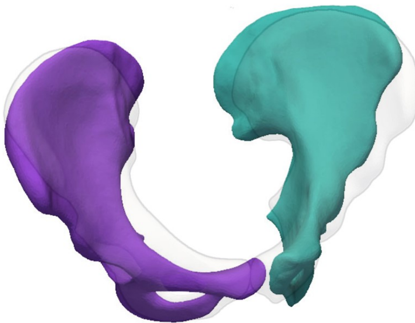
Fig. 33: Deformation of the pelvic bone model in first (purple) and second (green) modal stiffness.
