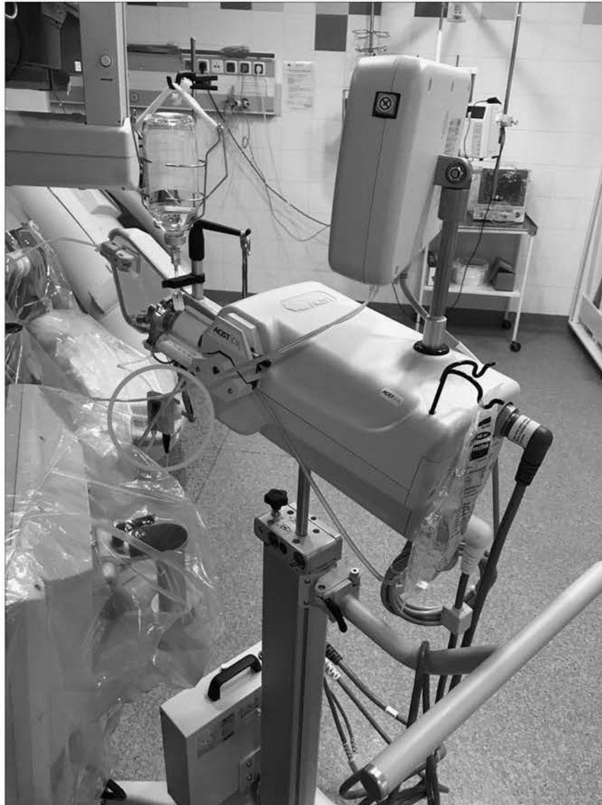
Figure 4. When using stand-alone (i.e. not mounted to the table) contrast medium injector, such as Acist CVI, pressure transducer must be recalibrated each time the patient is moved up or down so the transducer stays at the level of patient's heart.
