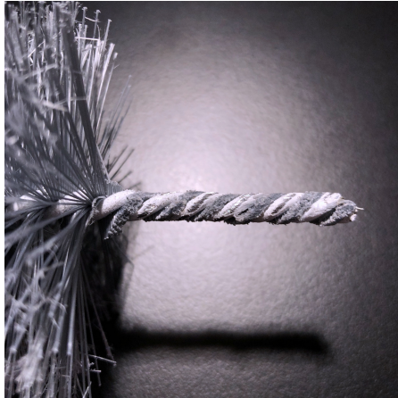
Figure 6.21: Cut and sanded steel core of the brush.
