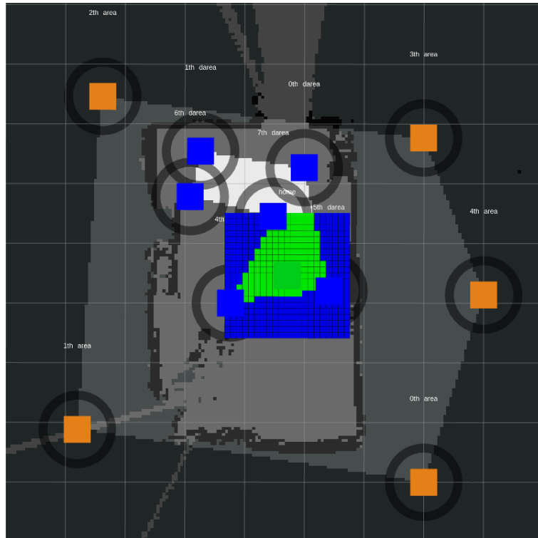
Figure 6.52: Points in a grid around home position, queried if they lie in the detection area.
