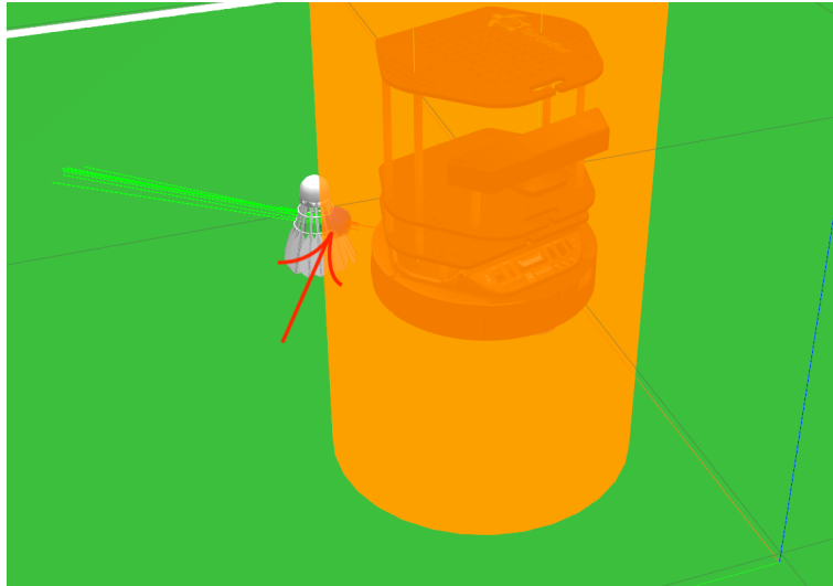
Figure 6.16: Contacts (pointed by arrow) detected between shuttle model and collision element (in orange).
