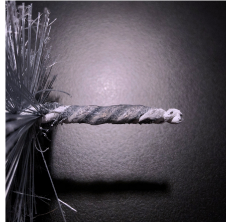
Figure 6.22: Brush after applying hot glue to the core.
