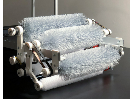
Figure 6.18: Finished, working prototype of picking mechanism.
