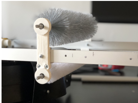
Figure 6.38: Drilled holes for fixed position.
