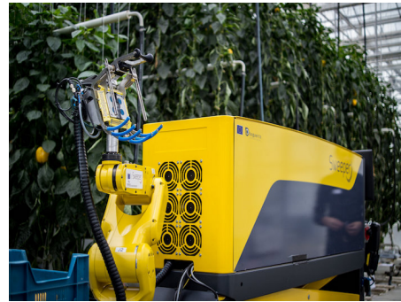
Figure 3.10: Closeup of end manipulator
