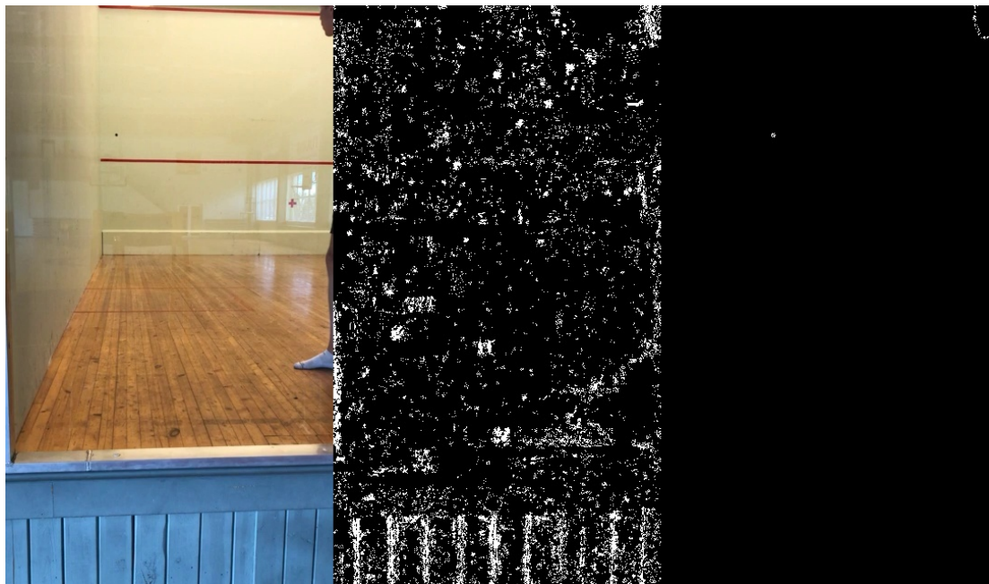
Figure 4.3: Regular frame (left), Otsu thresholded frame (middle), overridden thresholding(right).
