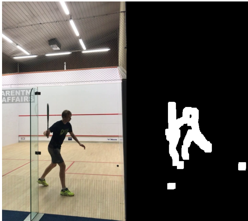
Figure 4.4: Normal frame (left) and extracted foreground from the background with two ball candidates(right).
