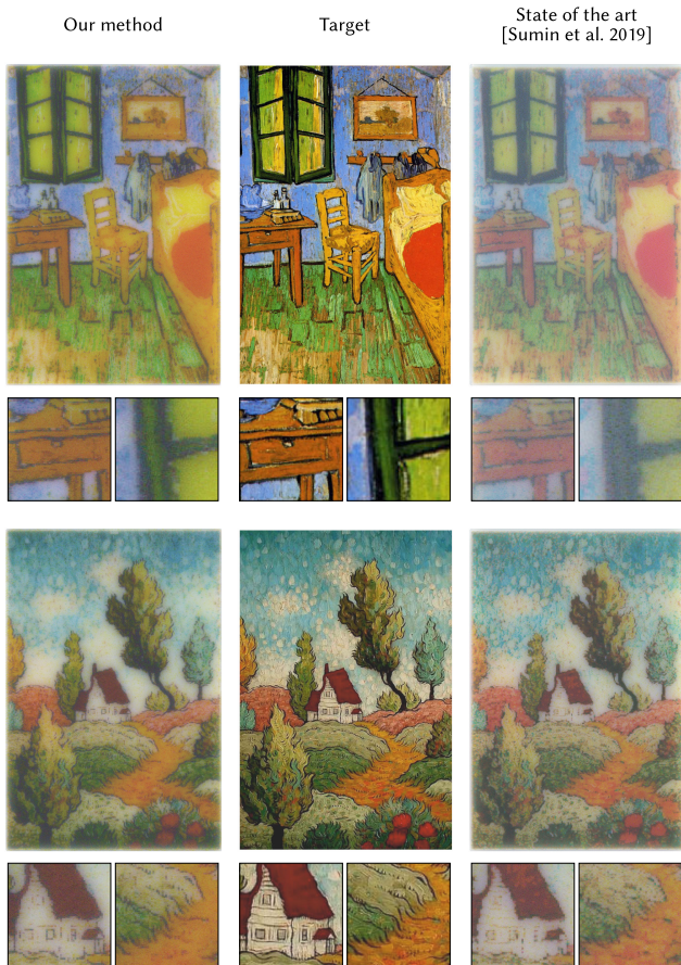
Fig. 9. Comparison of our results (left) to the state of the art (right) [Sumin et al. 2019] for a 2.5D planar slab, which has a different texture on each side. The slab is 30x20 mm large and 2.5 mm thick. Top: On the first side of the slab, our method achieves a significantly better color accuracy, saturation, and contrast than the state of the art. Bottom: The differences on this side are more subtle: our result overall appears “smoother” and managed to reproduce the dark edges better.
