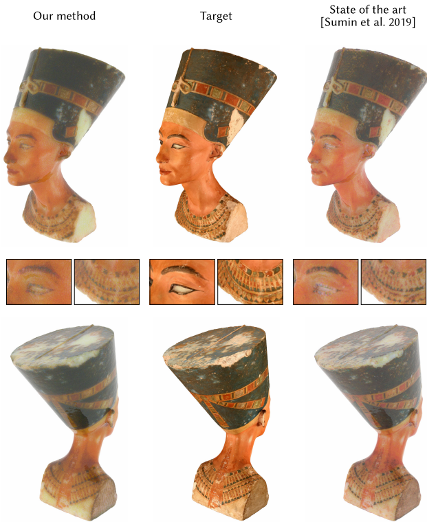
Fig. 10. A 4 cm tall reproduction of a 3D-scanned model of Nefertiti. Difficult areas are the eye region, where our method shows better detail, and the necklace, where Sumin et al. [2019] excels in contrast
