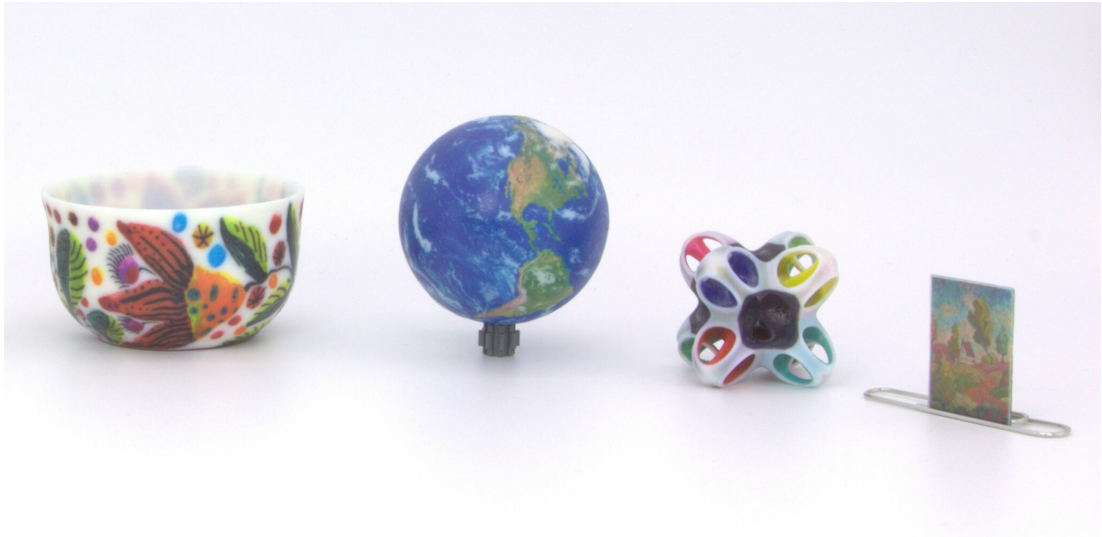
Figure 1.18: Photograph of some Polyjet printouts. The diameter of the globe is 6cm. Image by Sumin et al. [2019]
