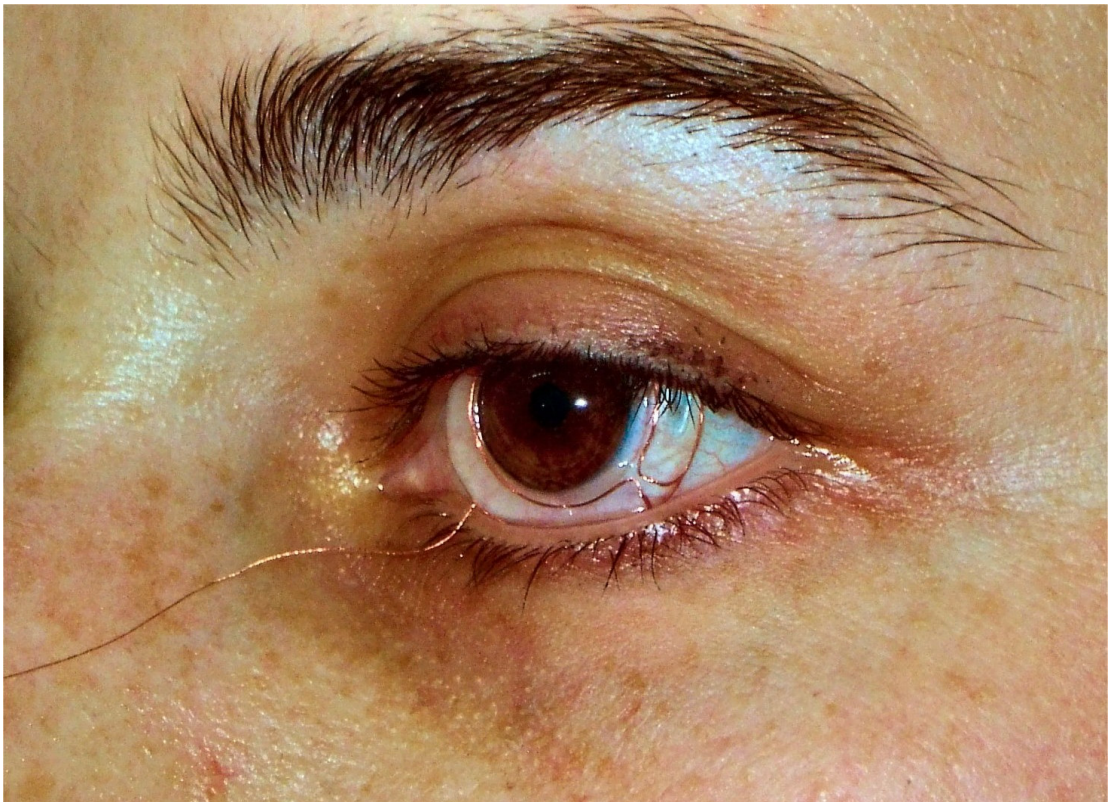
Figure III-4: Dual eye search coil placed in the eye. Coil is constructed of a contact lens containing a fine coil of wire, with leads coming out on the side, was placed in the subject's left eye after anesthetization of the conjunctiva with Oxybuprocain-HCl.
