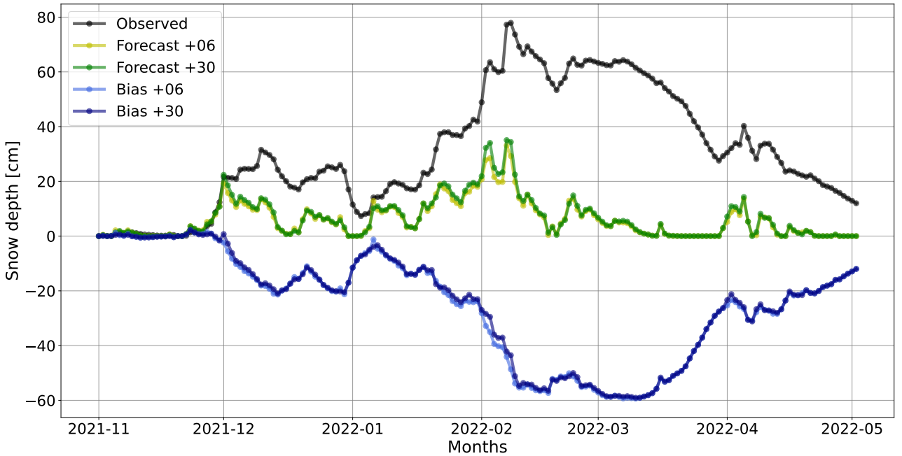
Figure 3.5: Time series of daily snow depth measurements, forecasts and their absolute bias for all regularly measuring stations in mountain altitudes
