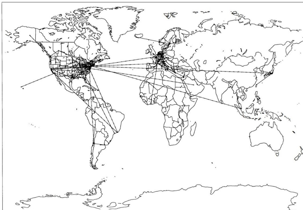
FIGURE 11 BITNET Connectivity Worldwide Source: Princeton University at Mon Oct 2 13:37:54 1989. netmap-1.5 program by Brian Reid, map data from World Data Bank II Gall Stereographic Projection—map center: [15°N, 0°W]. Image resolution 300/in., stroke limit 5 pixels.
