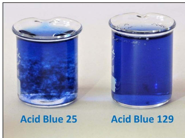
Fig. 6. Aqueous solution of Acid Blue 25 precipitates after acidification with hydrochloric acid and affords the templates (left) while Acid Blue 129 remains soluble (right).
