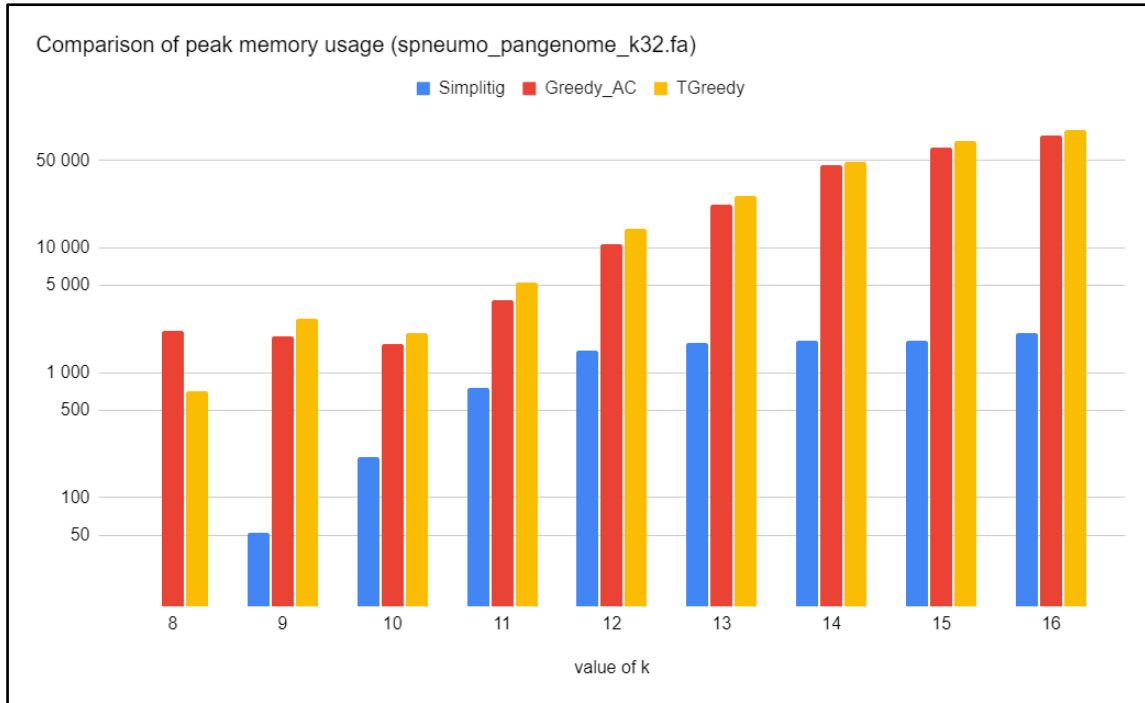
Figure 4.6: Comparison of the peak memory usage of algorithms Simplitigs, Greedy_AC and TGreedy for the value of k (range 8 - 16) and input file: spneumo_pangenome_k32.fa
