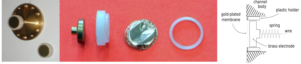
Figure 1.14: Photo (left) and scheme (right) of capacitive second sound sensor consisting of brass electrode and gold-plated porous membrane.
