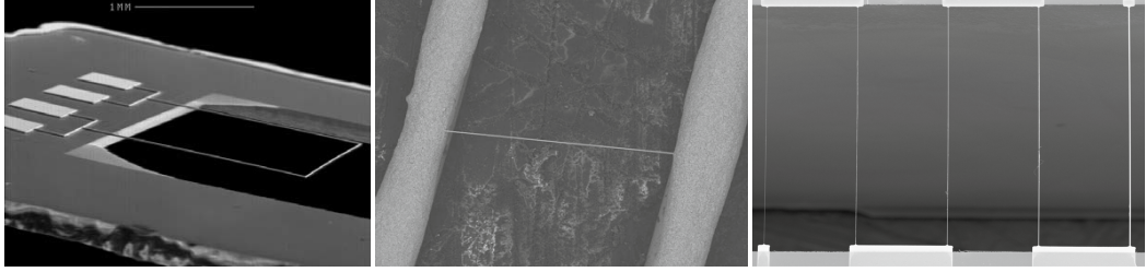
Figure 1.16: Illustrative photos of chosen mechanical resonators of micro- and nano-metric dimensions fabricated with use of lithography and other cleanroom processes. For more details see [27, 31, 149].
