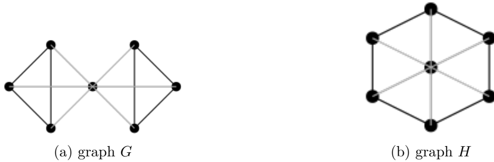
Figure 2.13: Classical example of graphs indistinguishable by 1-dim WL but distinguishable by \{2, 3\} -gdd
