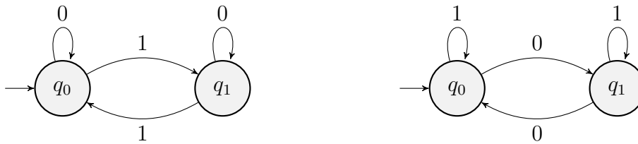
(a) Automaton discerning parity of ones (b) Automaton discerning parity of zeros
