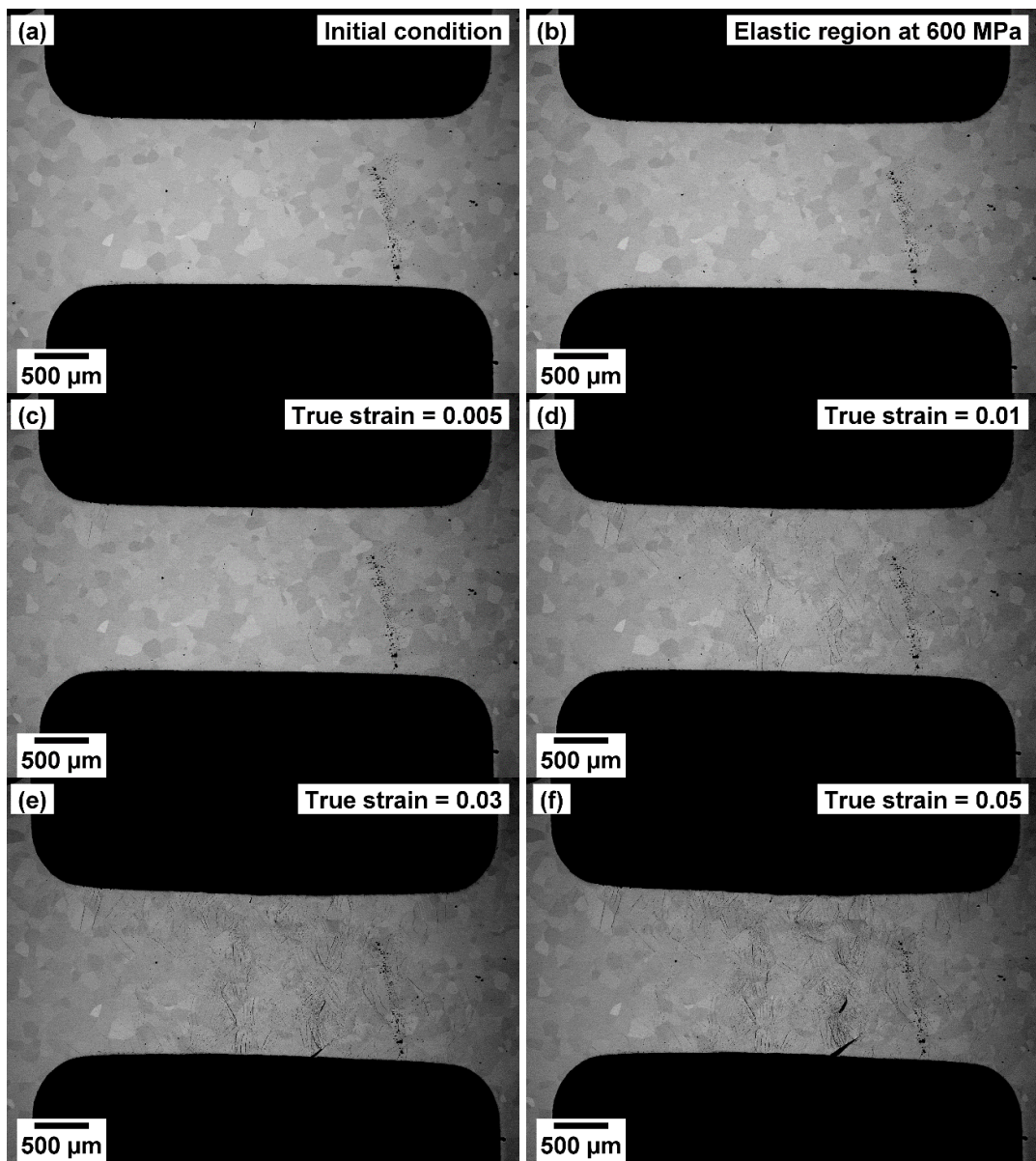
Figure 71: An overview of SEM images captured at various stages of tensile deformation. The crack formation can be noticed at true strains 0.03 and 0.05.
