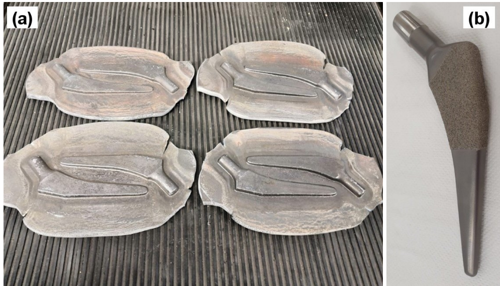
Figure 20: a) Implant semi-products formed by die forging from the swaged and solution-treated rod. b) Finished implant stem made from Ti-35Nb-7Zr-6Ta-0.7O alloy.
