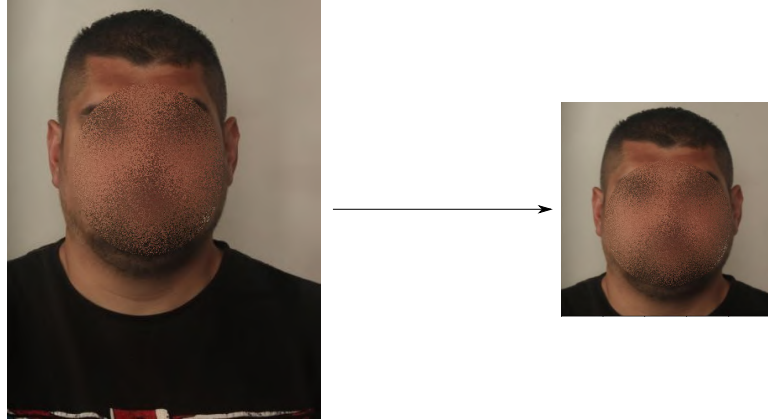
Figure 3.5: The result of cropping and then padding a face image where the left image represents the original image from which the face was cropped then padded and resized to 256 \times 256 pixels. Notice that in the original image, the face is in the top left corner of the image, while in the output image, the face is properly centered, both vertically and horizontally. The noise was added intentionally to the images for the sake of anonymization.
