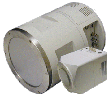
Figure 4.10: X-ray camera for the measurement of beam profile.
