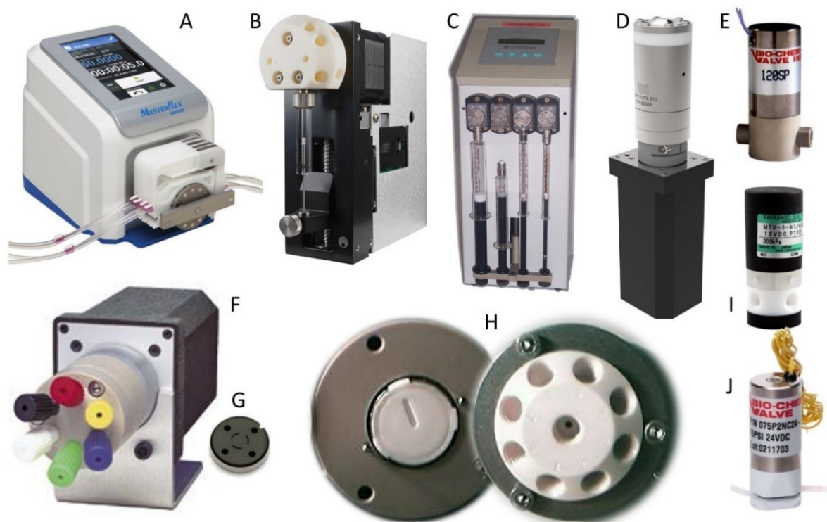
Figure 2: Pump and valve instrumentation used in flow analyzers: A: multichannel peristaltic pump, B: automatic syringe pump (with multiposition head valve), C: multisyringe pump, D: MilliGat® pump, E: solenoid pump, F: computer-controllable low-pressure injection valve with shown rotor (G), H: multiposition selection valve rotor (left) and stator (right), I: solenoid 3-way valve, J: pinch valve.
