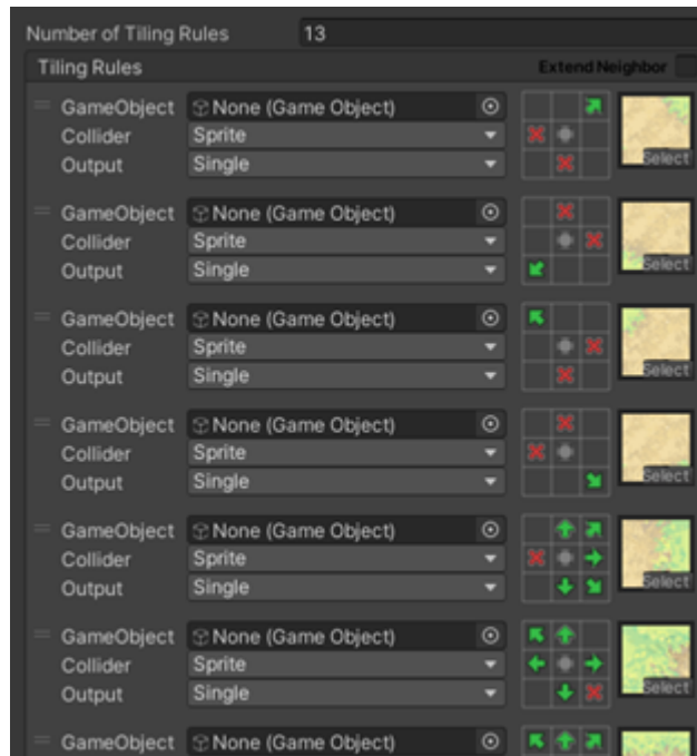
Figure 5.5: Land Rule tile gets defined by a set of rules. Each rule is described by a 3x3 grid representing the tiles around. Different markings in the grid represent different constraints: empty space, cross, or arrow corresponds to the position/edge where the tile can, can not, or should be connected to the other neighbor tiles.
