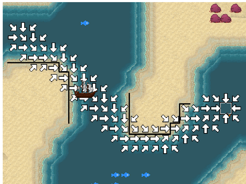
Figure 5.15: Ship's vector field for Water pathfinding. This field gets created from the A* generated list of tiles representing the shortest path to the destination. If any tiles from the list have neighboring Land tiles, the vector forces pushing from that Land tile get added to the Ship's vector field.
