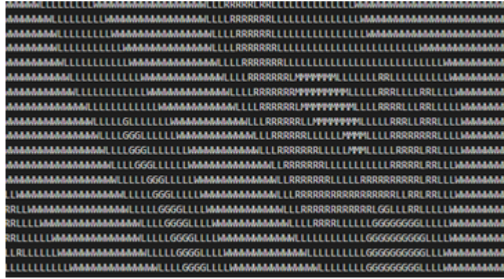
Figure 5.9: Map text file representing W character for Water tiles, L for Land tiles, R for RoughTerrain tiles, the G for Grass tiles, and R for MineralDeposit tiles.
