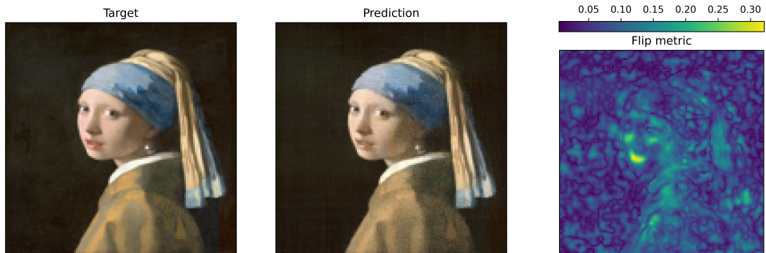
Figure 5.1: Result of 2D image representation network. The left image is the target, the middle image is the representation network output and the image on the right is the flip metric.
