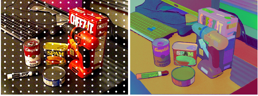
Figure 3.2: Example of image segmentation using SAM. Given an input image and a grid of point prompts (left), the Segment Anything Model retrieves the object mask for every point of the grid. The masks are then filtered by stability and confidence score, and duplicate masks are removed by NMS, resulting in the final segmentation of the image (right).
