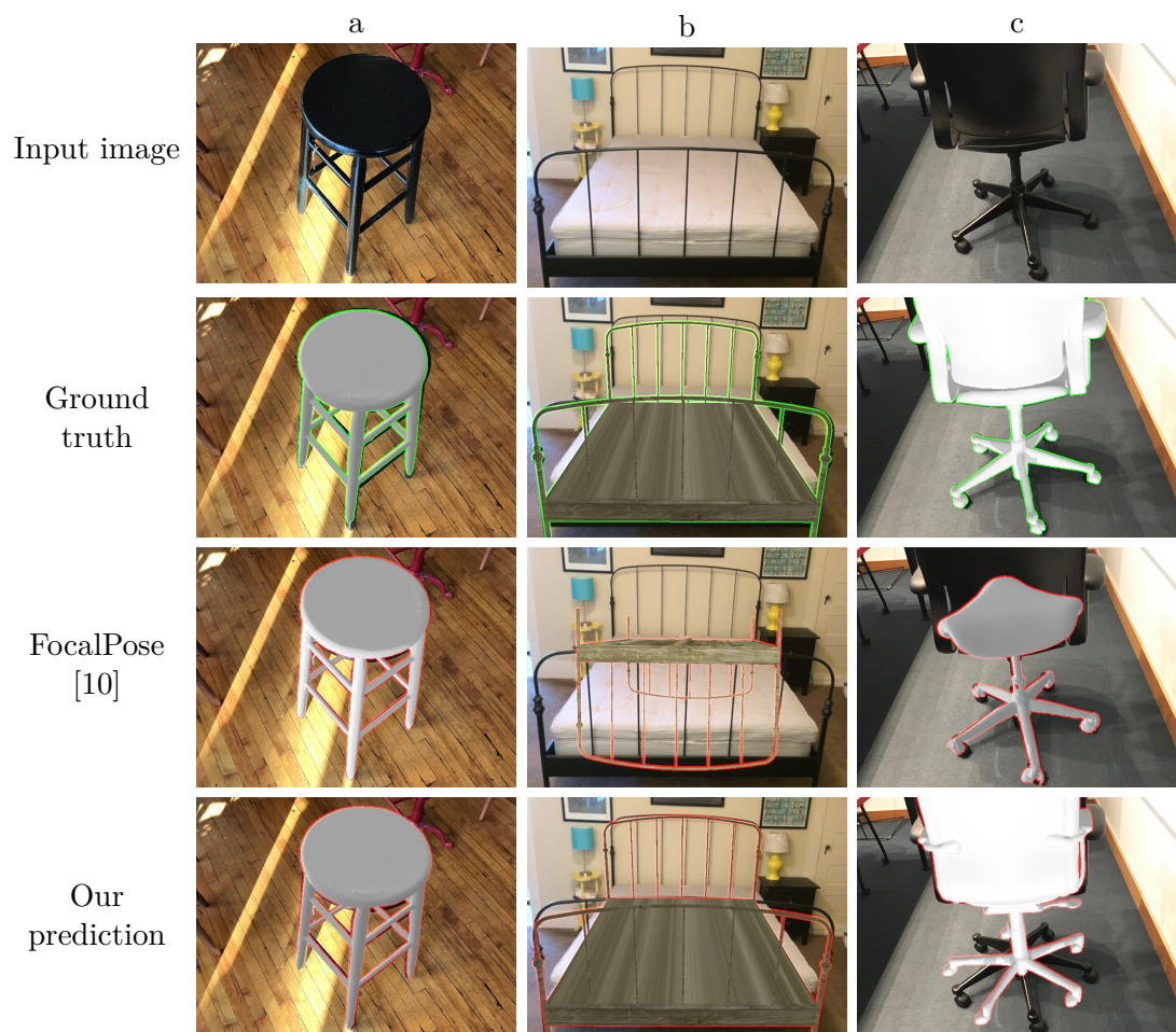
Figure 2.5: FocalPose main failure modes are: (a) symmetric objects, (b) local minima, and (c) incorrect 3D models identified by the object detector.
