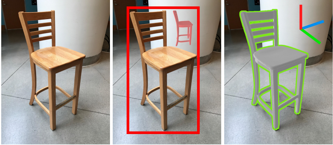
Figure 1: Typical model-based 6D pose estimation pipeline. Given an image of an object (left) and a database of 3D models, the task is to estimate camera-to-object 3D rotation and 3D translation. A typical pipeline consists of two stages. In the first stage (middle), a bounding box of the object is obtained and the 3D model of the object is retrieved from the database. Then in the second stage (right), the 6D pose of the object is estimated.
