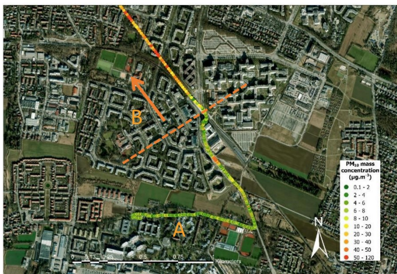
164 Fig. S5: PM_{10} variability (1 Hz) during the walk from the University campus to the subway station NS-U/S along 165 the main street with higher traffic (A), waiting on the over-ground platform open to the ambient air and a ride into 166 the tunnel by the old train (U5 line) with opened windows (B), 17. 5. 2022, 13:18 – 13:49
