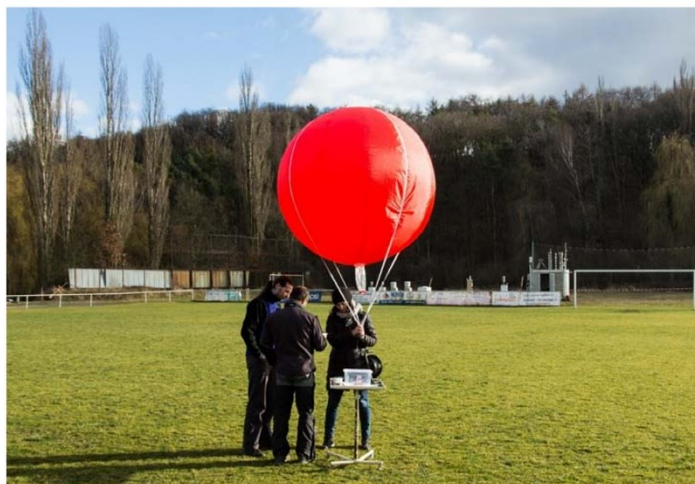
Figure 1. Tethered helium filled balloon for T and RH vertical profiles, air quality station in the background, Kladno-Svermov, Czech Republic, 6. 2. 2016
