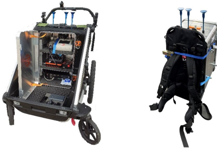
Fig. S1: Photo of the stroller (left) and the frame-rucksack (right) arrangement for walking measurements in the subway and used for other mobile aerosol measurements
