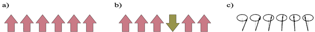
Figure 1.4: a) The classical picture of the ground state of a simple ferromagnet. b) A possible excitation: one spin is reversed. c) The low-lying elementary excitations, spin waves. The ends of the spin vectors press on the surfaces of cones, with successive spins advanced in phase by a constant angle (10).
