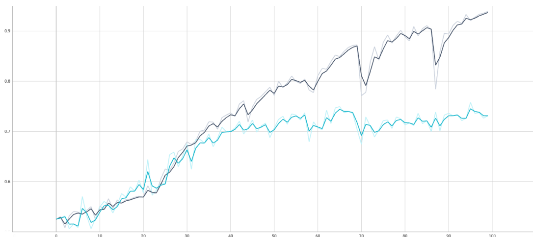
Figure 5.4 Training (black) and test (blue) accuracy of the Planar GNN on the NCI109 dataset, trained for 100 epochs
