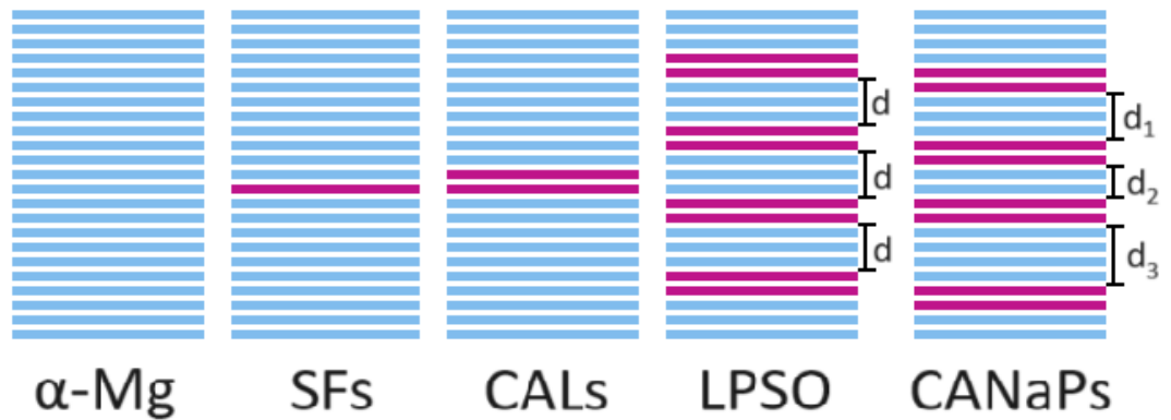
Figure 1.7 Illustration of \alpha -Mg lattice structure with SFs, CALs, LPSO, and CANaPs, where lines represent basal planes of the hcp structure
