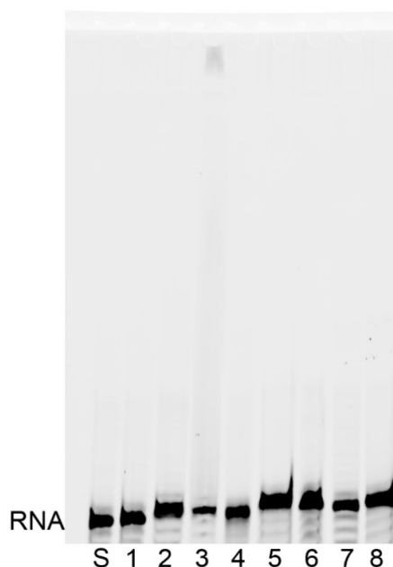
Figure 37. 22.5% dPAGE analysis of bioconjugation reaction of natural 21RNA_1A-Cy5 with (bio)molecules and various peptides. Gel legend: (S, RNA) natural RNA (21RNA_1A-Cy5), standard; natural 21RNA_1A-Cy5 in reaction with: (1) 10000 equiv. of reduced glutathione (GSH); (2) 10000 equiv. of pept-(+)-H; (3) 2500 equiv. of pept-(+)-C; (4) 2500 equiv. of pept(-)-C; (5) 10000 equiv. of Bio-thiol; (6) 10000 equiv. of FL-thiol; (7) 10000 equiv. of pept-K; (8) 10000 equiv. of pept-R. Cy5 channel scan.
