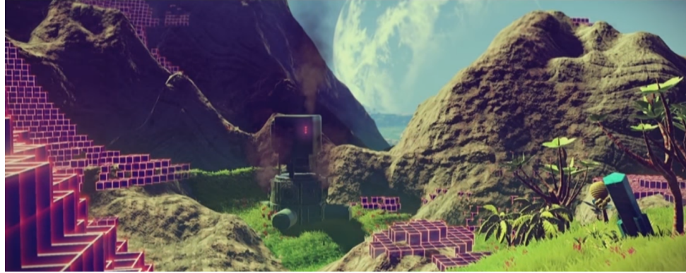
Figure 3 No Man’s Sky generated environment generated using voxels and polygonised using Dual Contouring and Marching Cubes algorithms. [10]
