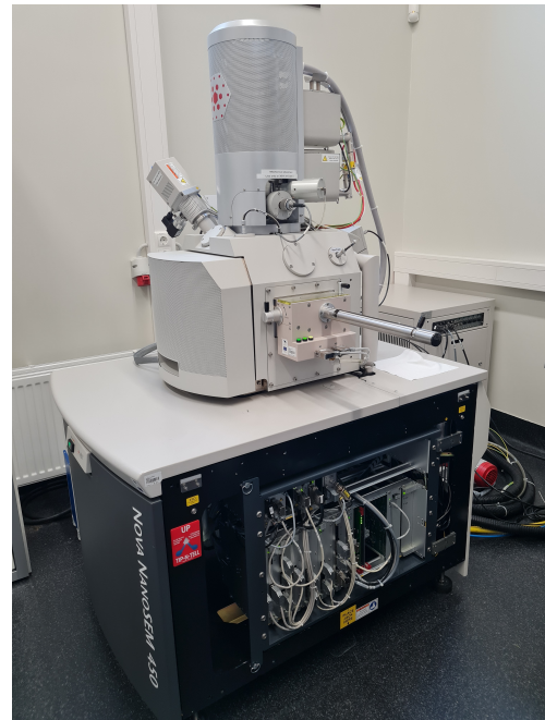
(b) FEI Nova NanoSEM 450 located at the Institute of Physics, University of Tartu used for heat-treatment measurements.
