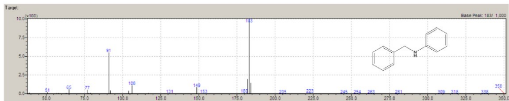
Figure 80: GC-MS spectra of N-benzylaniline, 48 h test
