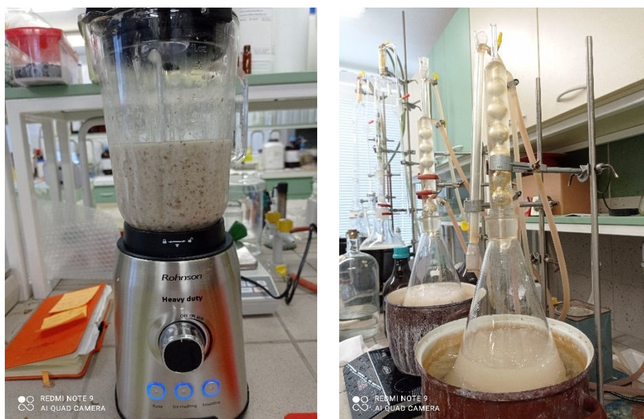
Figure 14. Bulbs processing. Mincing of bulbs with 96% EtOH (left) and heating a suspension under reflux (right).
