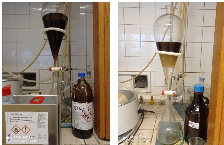
Figure 15. LLE after basification with EtOAc (left), and CHCl 3 (right).
