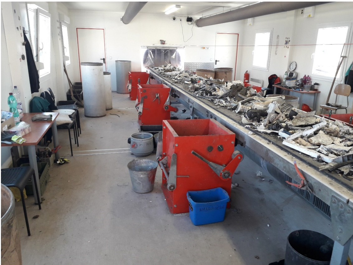
Figure 5 The conveyor belt at the sorting line.
