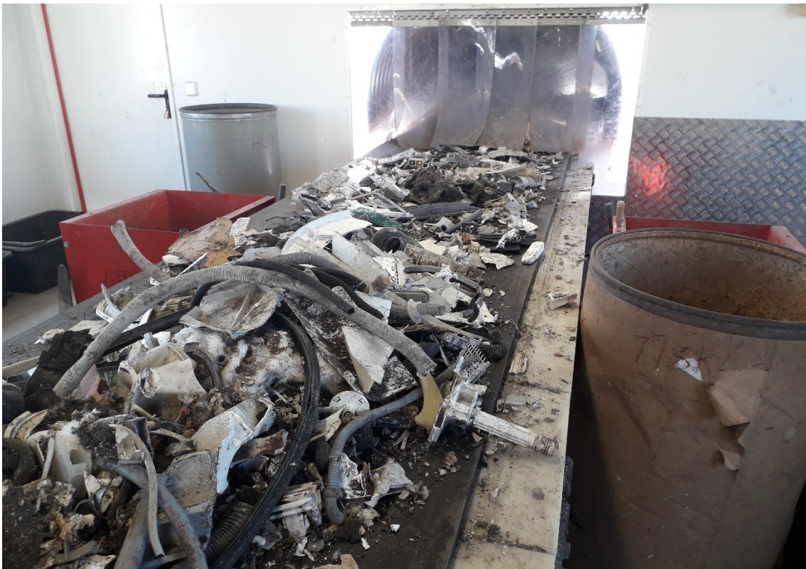
Figure 8 The mixture of various e-waste parts at the sorting line.
