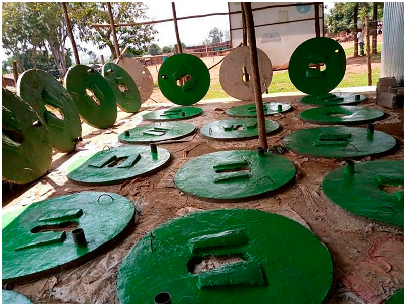
Figure 3. Prefabricated cemented slab platforms available nearby to the study area. Sources: The authors.
