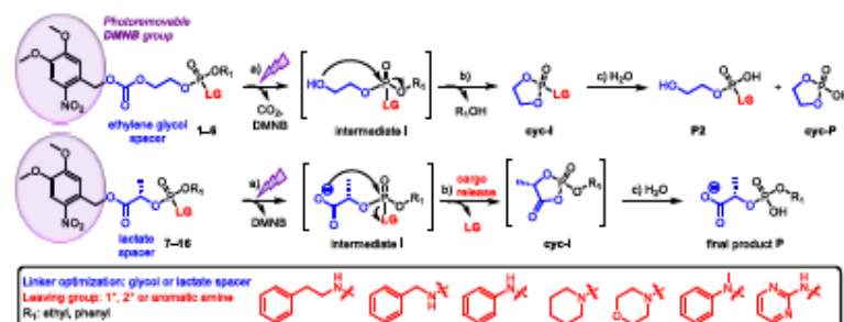
Figure 1. Self-immolation (SI) of 1–16; (a) SI is initiated by UV light (365 nm), which cleaves a photosensitive DMNB group [21]; (b) the intermediate I then spontaneously cyclizes, releasing R_1 (4–6) or LG (7–16); (c) hydrolysis of the lactate-based cyclic intermediate leads to the final product P, whereas glycol-based cyc-I hydrolyzes to the final product P2 or the cyclic product cyc-P .
