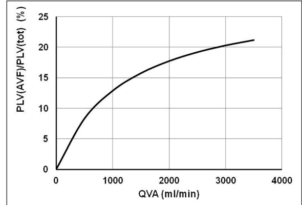
Figure 3. Relative part of the whole power exerted by the left ventricle to run the blood flow through the VA ( P_{LV}(AVF)/P_{LV}(tot) ) as a function of QVA as defined by equation (11).
