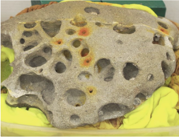
Figure 6: A testing of evaporation dynamics on a metasandstone block with honeycombs. The block is placed in a plastic dish with a piece of cotton cloth, which serves as a capillary water inflow path to the block. Narrow drill holes to measure the depth of the evaporation front are highlighted by an orange zone of uranine dye (Mareš et al., 2022).
