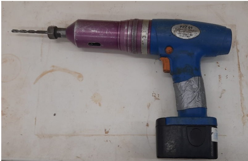
Figure 4: Drilling machine for testing drilling resistance.
