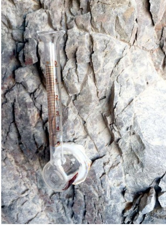
Figure 5: Measurement of the infiltration rate using Karsten tube (Mareš et al., 2024a).
