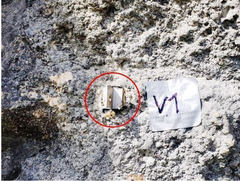
Figure 3: Measurement of tensile strength using pull-off test (Mareš et al., 2024a).
