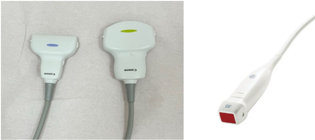
Figure 1 - Ultrasound probes: On the left is a linear probe, the middle is a curvilinear probe, and the phased array is on the right.
