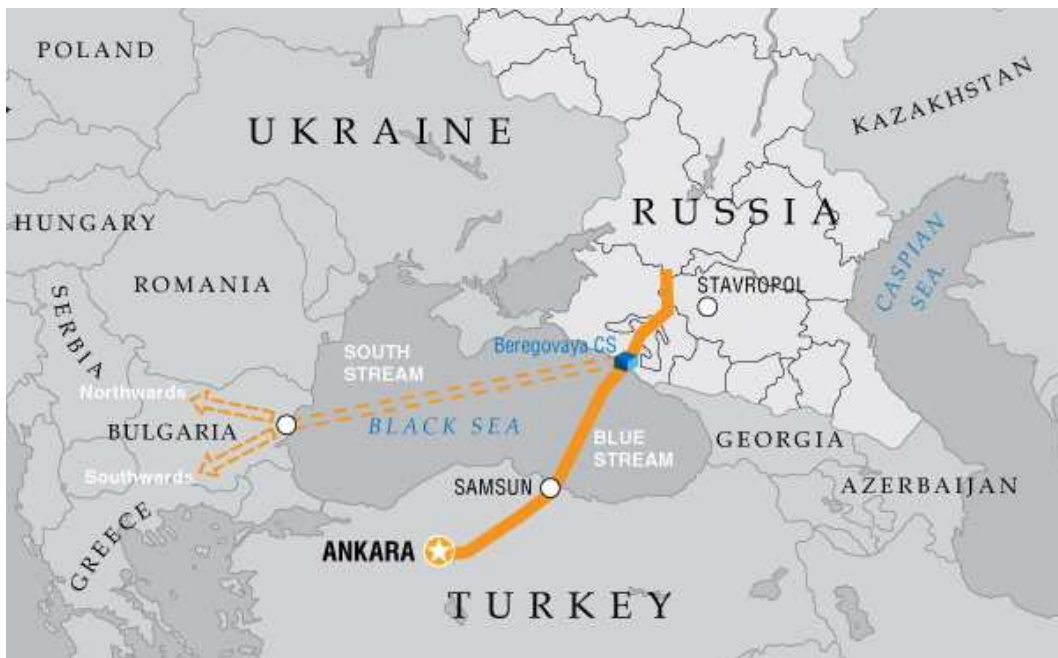
Figure 10: Blue Stream gas pipeline map
