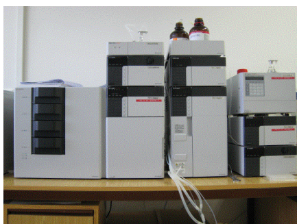
Obr. 80 HPLC set Prominence LC 20 (Shimadzu, Kyoto, Japonsko)
