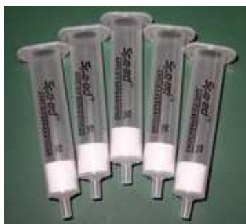
Obr. 75 Kolony Spe-ed C18 pro SPE extrakci
