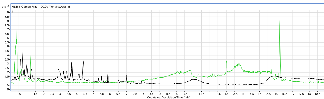
Figure 33: Amino acids standard, HILIC column (black line), F5 column (green line)
