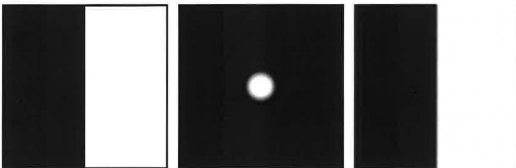
Figure 6.4: A smooth Fourier filter (middle plot) and a 2D step function (left plot). Filtering artifacts strongly present in Fig. 6.3 are reduced remarkably.
