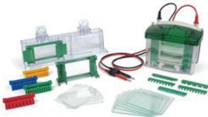
Fig. 5 Mini PROTEAN Tetra Cell system It contained short plates, plates of 1.5 mm, 15-well combs, casting stand with 2 casting frames, power supply with constant voltage.
