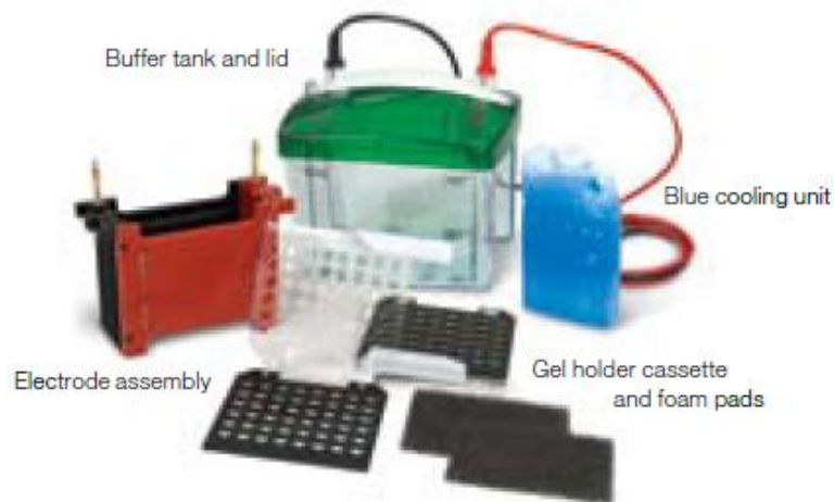
Fig. 6 Blotting system Mini Trans-Blot cell It contained buffer tank and lid, electrode assembly, cooling unit, gel holder cassette and foam pads.
