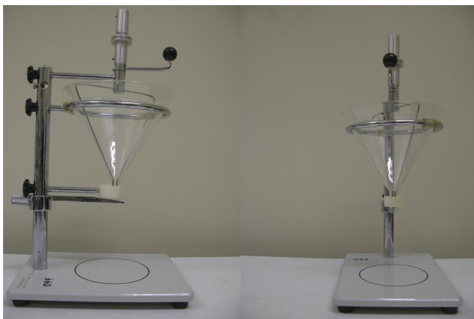
Figure 15: Device used for flowability measurements
