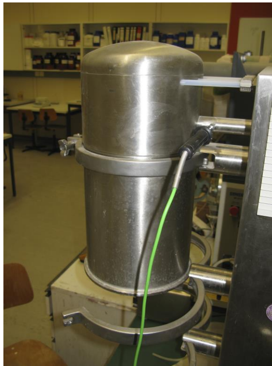
Figure 13: emplacement of thermo-probe for drying part of granulation
