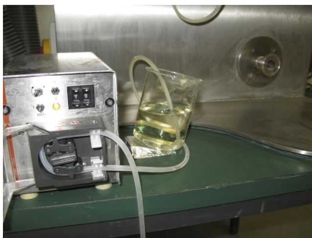
Figure 7: Binding solution prepared for granulation run
