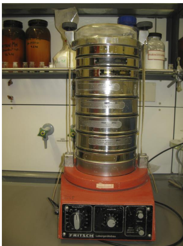
Figure 14: Sieving tower Retsch used for Particle size distribution analysis
