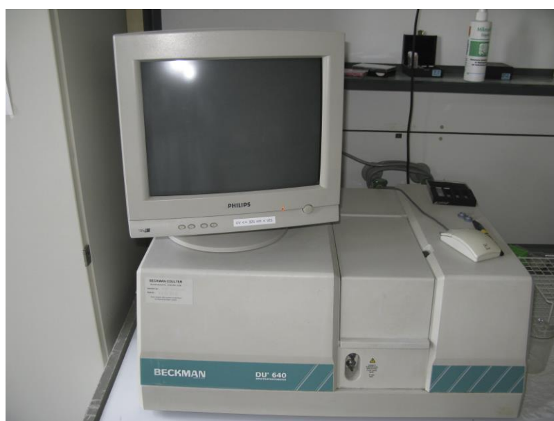
Figure 16: UV Spectrophotometer Beckman-Coulter Du® 640
