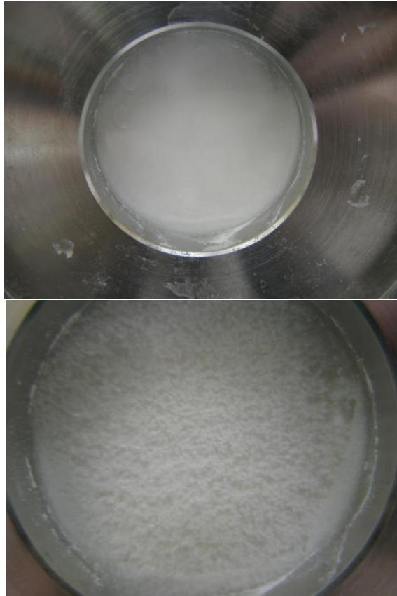
Figure 12: Particle growth over-watched through the round window of material container
