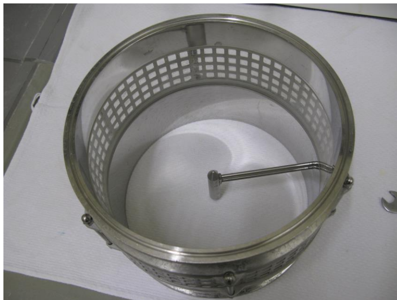
Figure 10: Spray housing part of granulation chamber with attached spraying nozzle in low distance top spray arrangement
